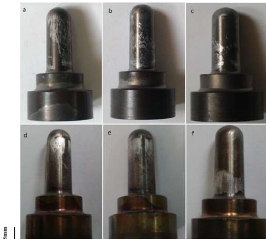
Figure 11 – Pictures of the Cr/CrN/CrAlN (a,b,c,) and Cr/CrN (d,e,f) coated pins after demolding test
