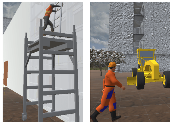
Figure 3. Left: An worker in a fall hazard situation. Right: An worker in a struck-by hazard situation.
