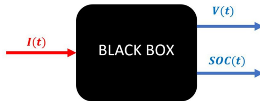
Fig. 30 Diagram of the approach used to apply the DM for the battery model
