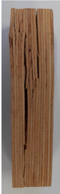
Figure 7: Parallel to the grain compression specimen failure
