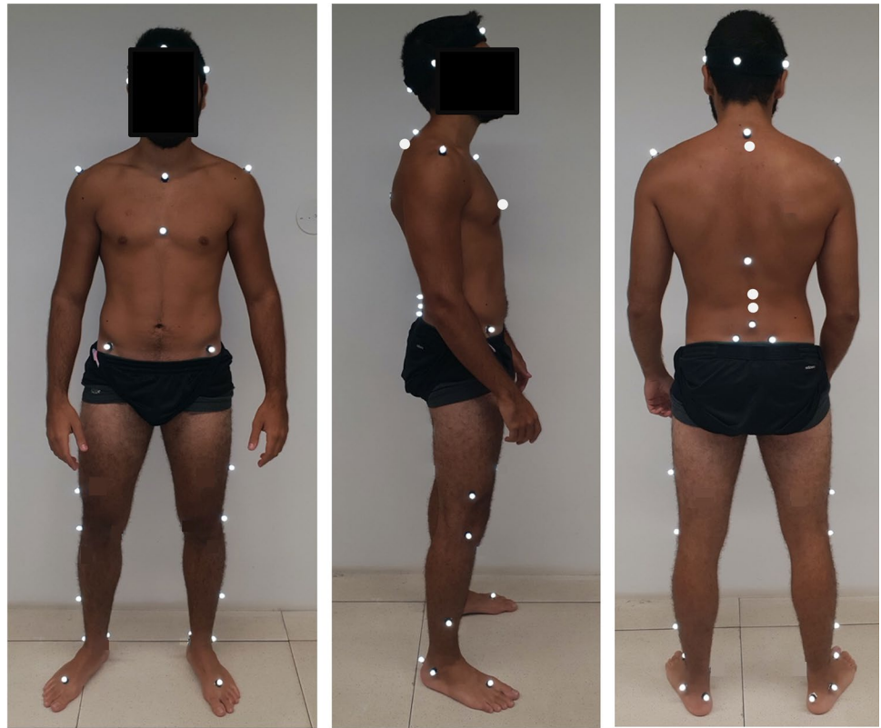
Fig. 1 Marker set for the modified Davis protocol (Plug-In Gait model) and Leardini protocol
