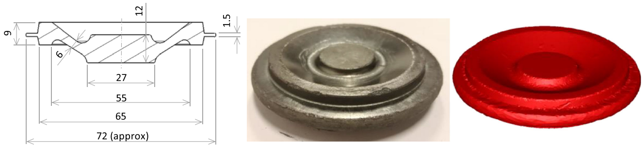
Fig. 13 Semi-industrial validation part: dimensions (left), experiment (center), simulation (right)
