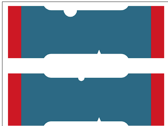
FIGURE 14 | Two different parameters configurations. Top: R = 7.59 , S = 18.23 , h = 0.84 ; bottom: R = 3.75 , S = 5.58 , h = 1.51 (all dimensions are provided in mm). The red zone is the part subject to rigid body constraints.
