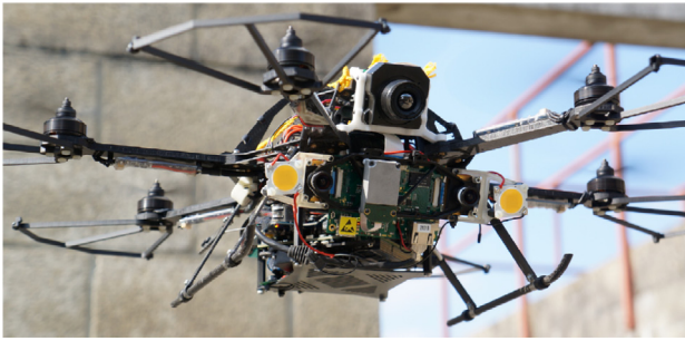
Fig. 20. Firefly UAV equipped with the VI sensor [41].
