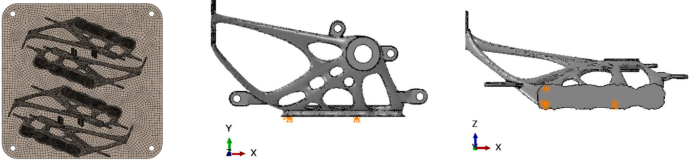
Fig. 19. Mesh of the nesting (left) and boundary conditions for the wire-cut step (right). The orange cones are the blocked degree of freedom. (For interpretation of the references to color in this figure legend, the reader is referred to the web version of this article.)
