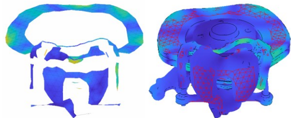
Figure 5 Squeal ODS (left) and expanded shape with \gamma = 1e4 (right)
