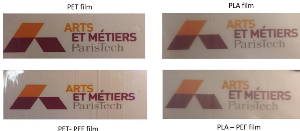
Figure 1: film sample of PET, PLA, PET-PEF and PLA-PEF
