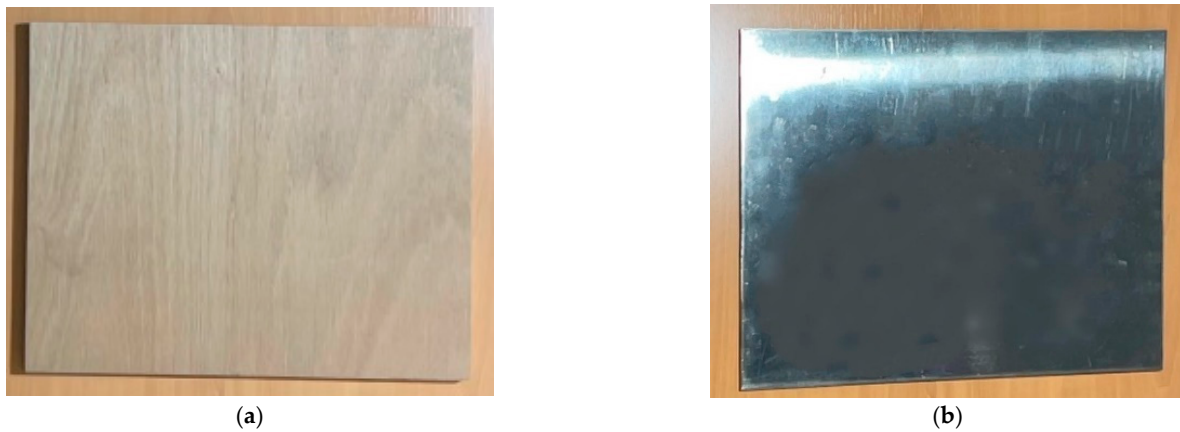
Figure 11. (a) Wooden plate (diffuse reflection) and (b) aluminium plate (specular reflection): the visual impact shows the strong light reflection of a specular surface compared to a diffuse surface.
