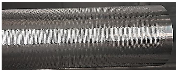
Fig. 2. A poor surface finish as an example for chatter.
