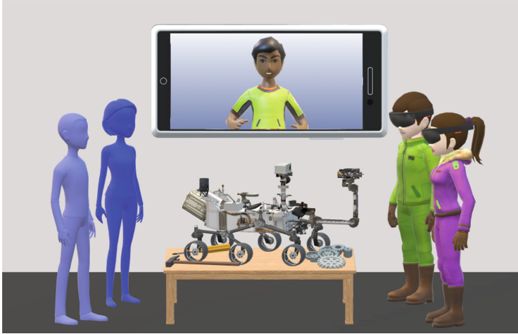
Fig. 2. Concept of a CVE with mixed collaboration modes and xR technologies. Left: Avatars of remote collaborators participating via VR HMDs or a CAVE. Center: Collaborator participating through a video call on their desktop PC or hand-held device. Right: Present (co-located) collaborators using AR HMDs. Source: own representation.
