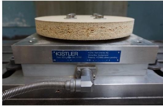
Figure 2. Peripheral milling setup used for the measurement of the cutting forces.
