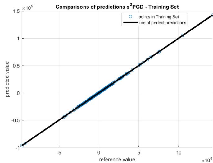
Fig. 11 Problem defined in Eq. 4.5: Comparison of predicted s^2 -PGD values with the reference ones in the training set (the black line represents a perfect prediction)
