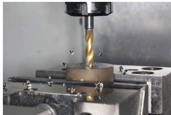
Figure 3. Experimental setup during the dry drilling tests.
