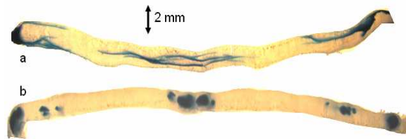
Figure 3: Morphology at the die exit for systems 2(a) and 3(b)
