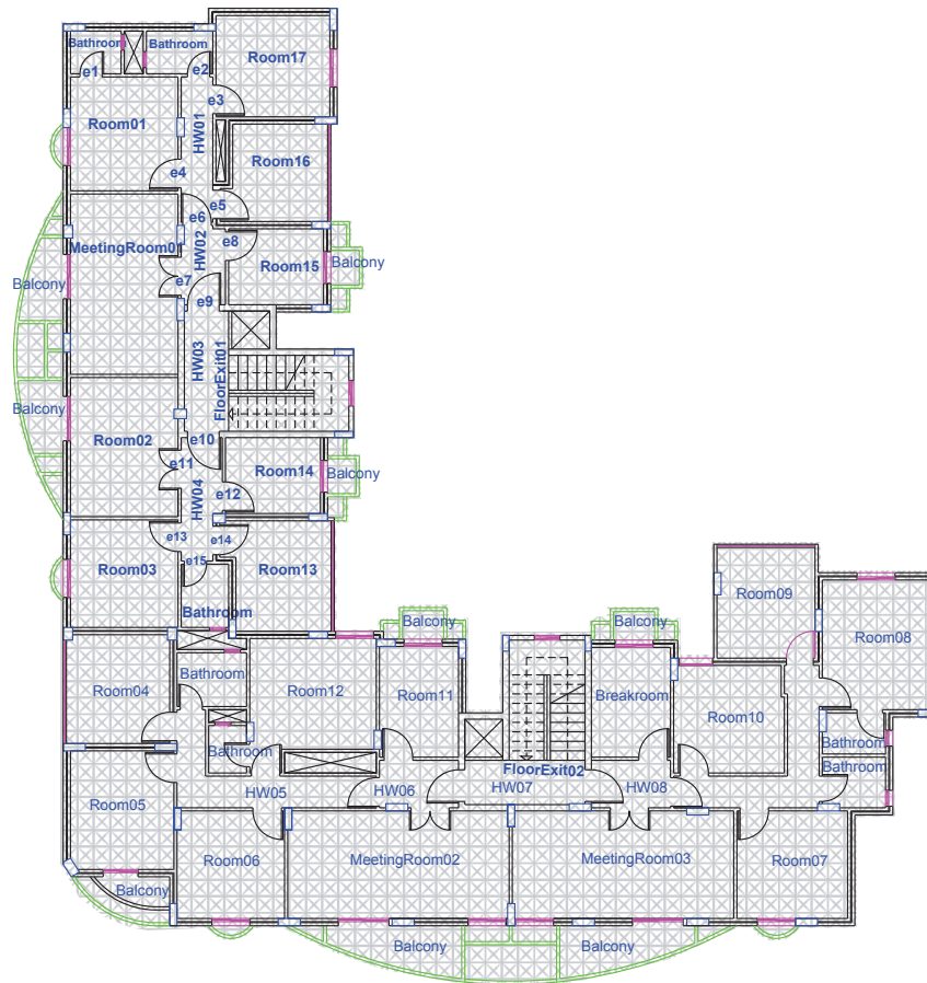
Figure 11: Example of a fine-grained graph of a floor plan.
