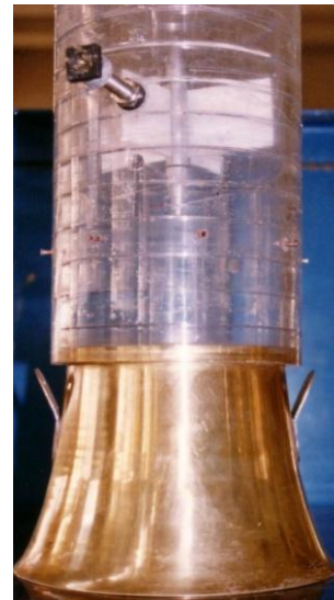
Figure 2. four-bladed swirl meter
