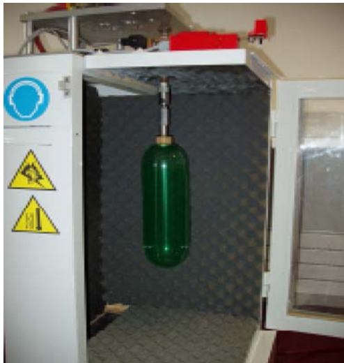
Fig. 4 Free-blowing test machine of preforms
