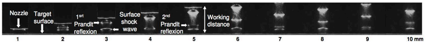
FIG. 5. Strioscopic images of the target surface for several working distances (WD) in millimeters with a 2 bars nozzle pressure.
