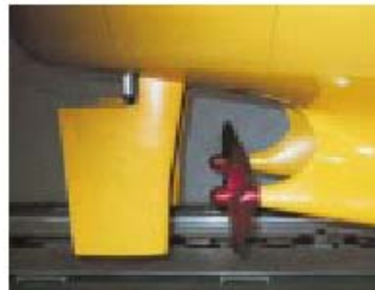
Picture 2. ULCS twin screw - twin skeg.
