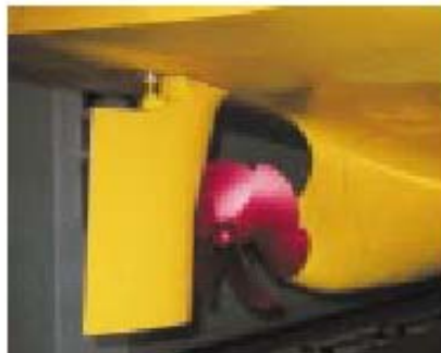
Picture 1. ULCS single screw - single skeg.
