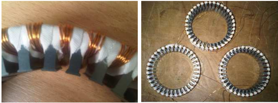
Figure 1: Samples of stators wound manually
