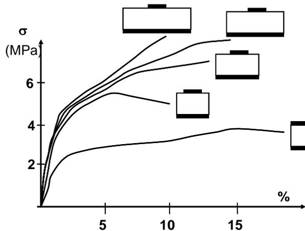
Figure 1. Compressive strength perpendicular to the grain
