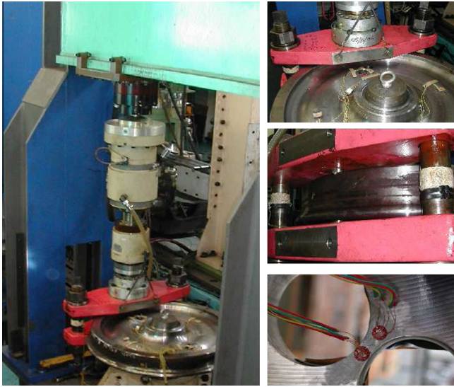
Fig. 14. Drilled wheel on SNCF-AEF fatigue test bench.
