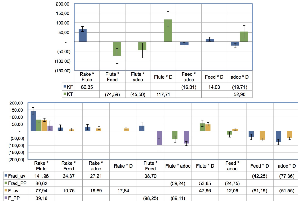
Figure 7: Representative Effects of Basic and Interaction Parameters on Specific Forces (on the upper bars), Radial and Resultant Average Forces, and Radial and Resultant Peak-to-peak Forces (on lower bars)
