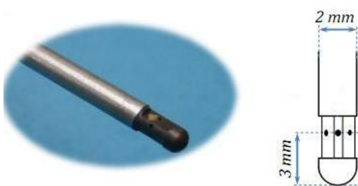
Figure 1. View of the directional probe
