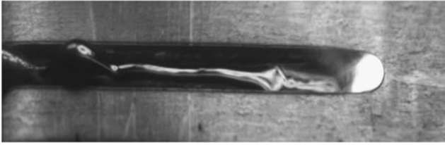
Fig. 9 Experimental observation of humps formation
