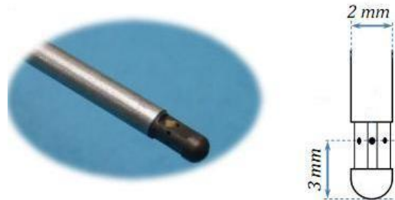
Fig. 1 Picture and sketch of the three-holes pressure probe
