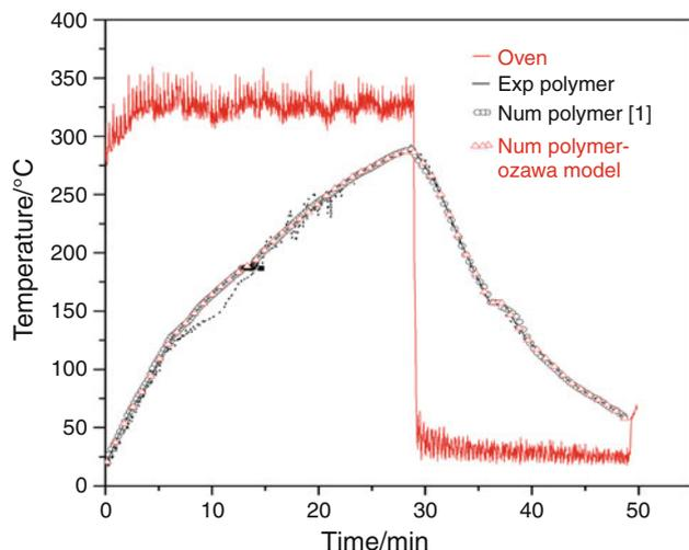
**Fig. 8** Temperature versus time ( $T/t$ ) diagram of PA11 according to enthalpy method (layer to layer), Ozawa model and experimental one
