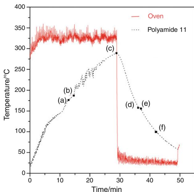
**Fig. 1** Temperature versus time, (T/t) diagram of PA 11. Various points indicate: (a) fusion of ‘elementary’ layer of polymer powder in contact with mould internal surface; (b) fusion of ‘elementary’ layer furthest away from mould surface; (c) end of heating and cooling beginning; (d–e) polymer crystallization; (f) end of rotational moulding
