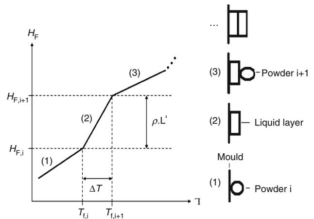
**Fig. 5** Enthalpy evolution law according to temperature. Main parameters are:  $T_{f,i}$  = initial fusion temperature of elementary layer ( $i$ );  $T_{f,i+1}$  = initial fusion temperature of elementary layer ( $i + 1$ );  $L'$  = fusion latent heat and  $\rho$  = solid polymer density
