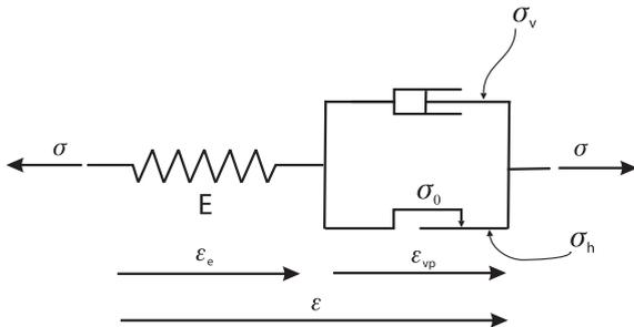
Fig. 1. Elasto-viscoplastic model.
