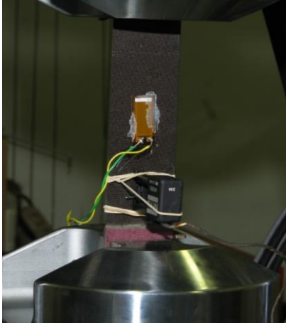
Figure 5: Tensile load of a monolithic specimen
