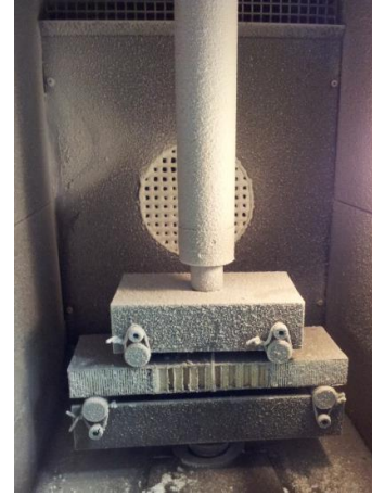
Figure 6: Flexural load of a sandwich specimen at -60°C
