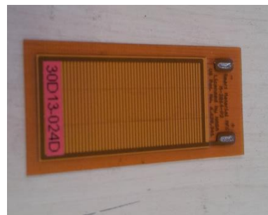
Figure 4: MFC patch from SMART-MATERIALS
