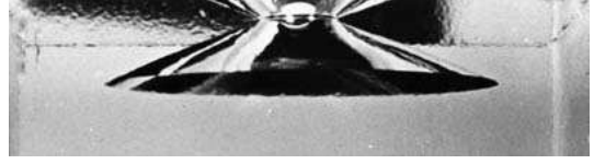
Figure 5: The hertzian cone; image taken from (30).
