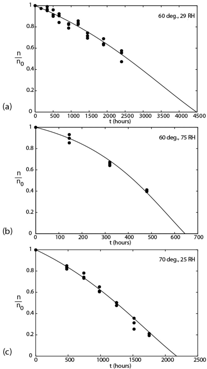
Figure 4. Crosslink density variation (relative units) against time of exposure at: 60°C, 29% RH (a); 60°C, 75% RH (b); 70°C, 25% RH (c) Symbols: experimental results. Curves: model (second approach).
