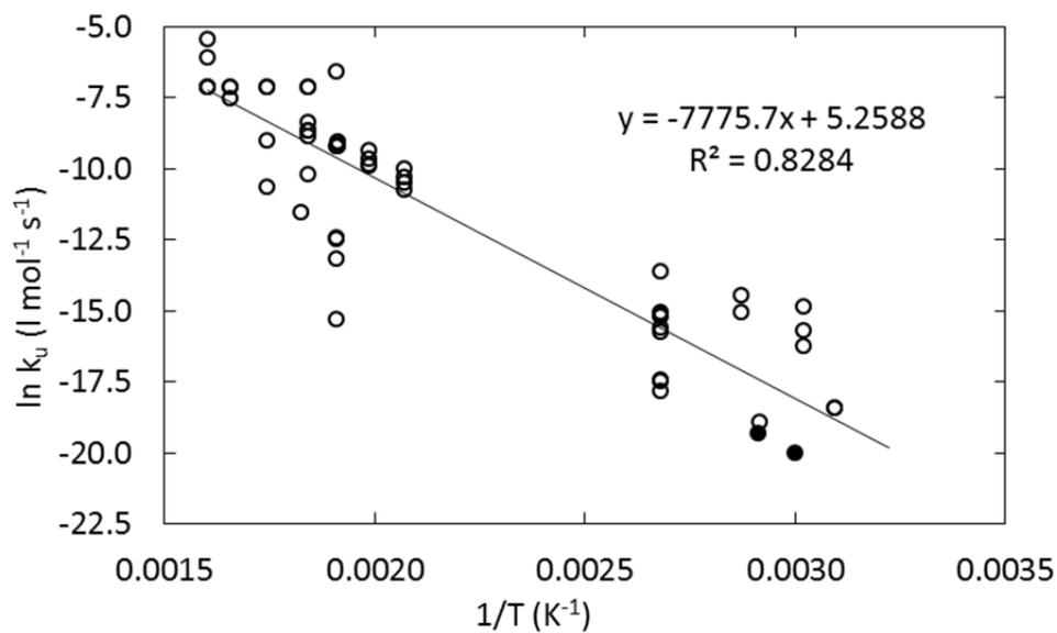
Figure 5. Arrhenius plot of  $k_u$  values from literature (○) and obtained in this work (●).
