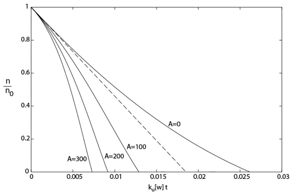
Figure 6. Reduced crosslink density against reduced hydrolysis time for  $L=18$  and several values of the autocatalysis ratio.
