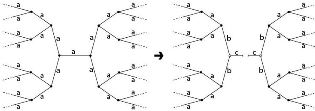
Figure 1. Illustrating scheme for the loss of three elastically active chains resulting from one chain scission.
