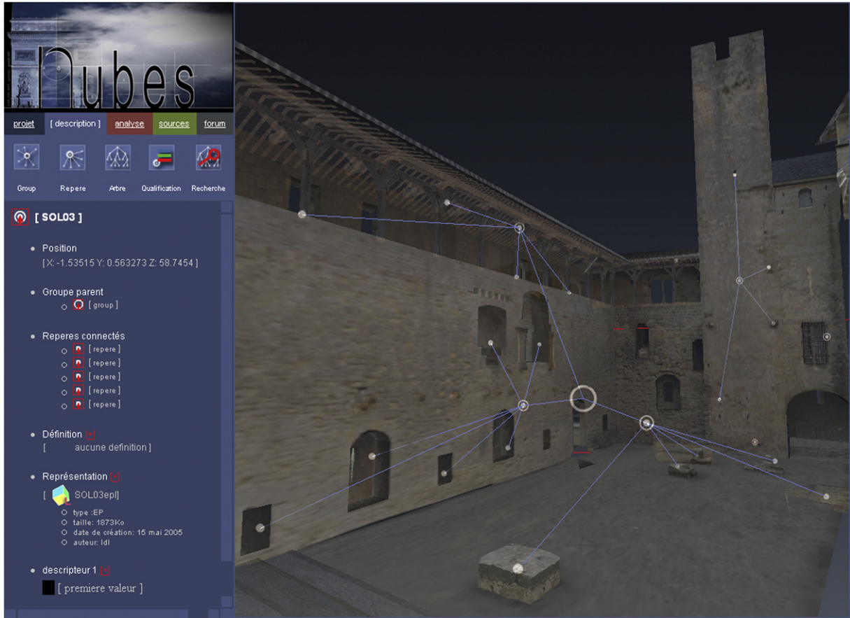
Fig. 7. Semantic qualification of a 3D representation in Nubes Visum. The user can select a morphological entity, assign a vocabulary term, choose a type of representation (point cloud, profiles, polygons, etc.), qualify entities by custom attributes and create related reference marks.
