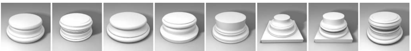
Fig. 22. Bases modeled by declaration of a sequence of mouldings
