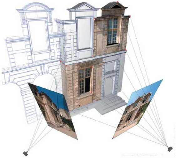
Fig. 17. The texture mapping process.
