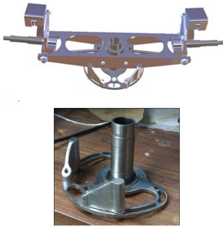
Figure 5: Forward steering part [LC1].
