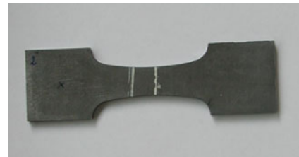
Fig. 3 Shape of the blanked specimen
