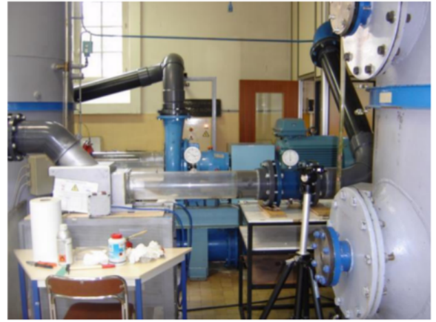
FIG. 4. Scheme of the DynFluid axial pump test-ring
