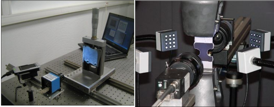
Fig.1. Fringe generation in the case (a) of projected fringes (courtesy of EMSE) (b) of the grid method (courtesy of Arts et Métiers ParisTech)
