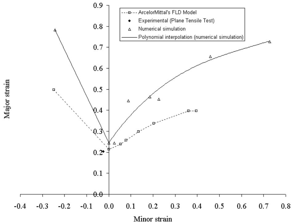
Fig. 13. Ellipticity loss simulations (ELDs) for a single phase steel for linear and complex loading paths.
