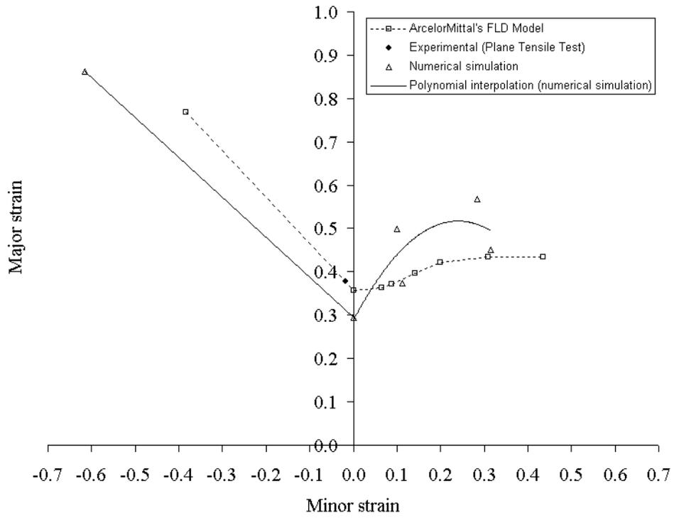
Fig. 12. Ellipticity loss prediction: comparison between direct ELD and ArcelorMittal's reference FLD for a dual-phase steel.
