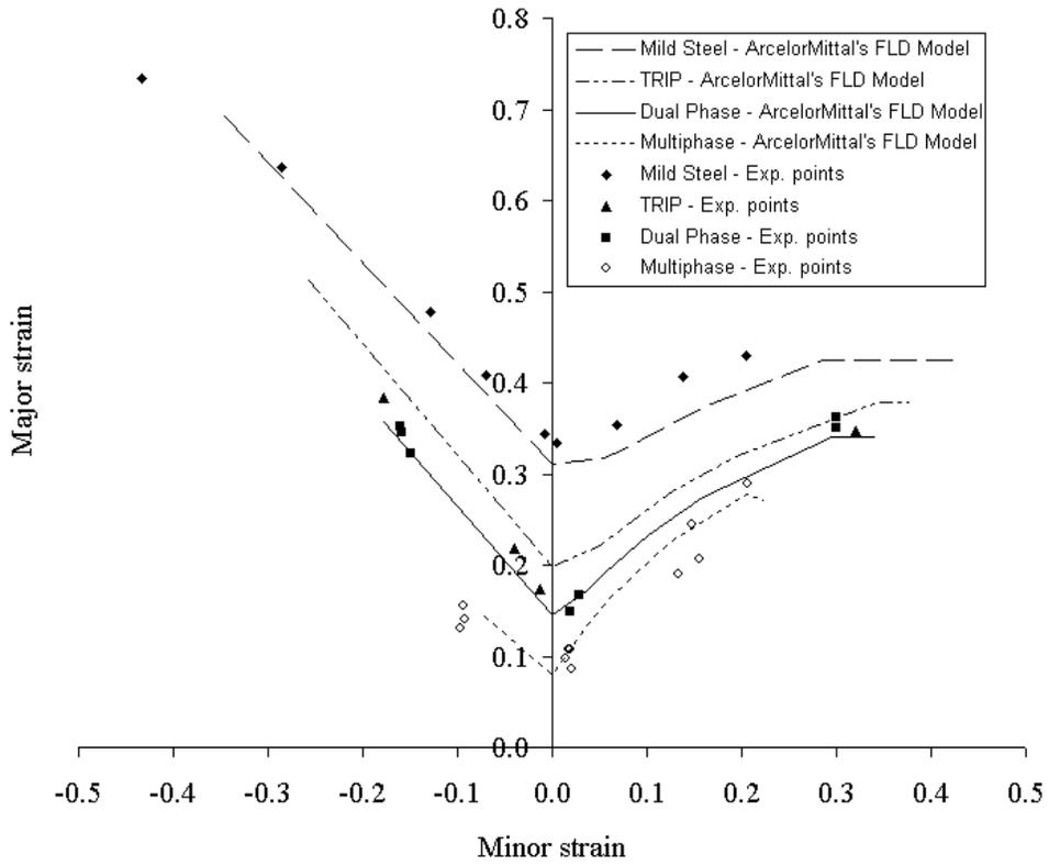
Fig. 11. Ellipticity loss prediction: comparison between direct ELD and ArcelorMittal's reference FLD for a single phase steel.
