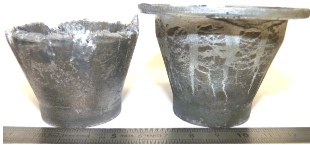
Fig.9 Parts thixoextruded at 590 °C and 620 °C
