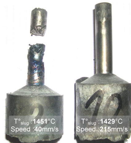
Fig. 17. Two thixoextruded parts having a bad shape (left) and an exact shape (right) forged at the same load (200 kN) but for different initial slug temperature and ram speed (“cold” die).
