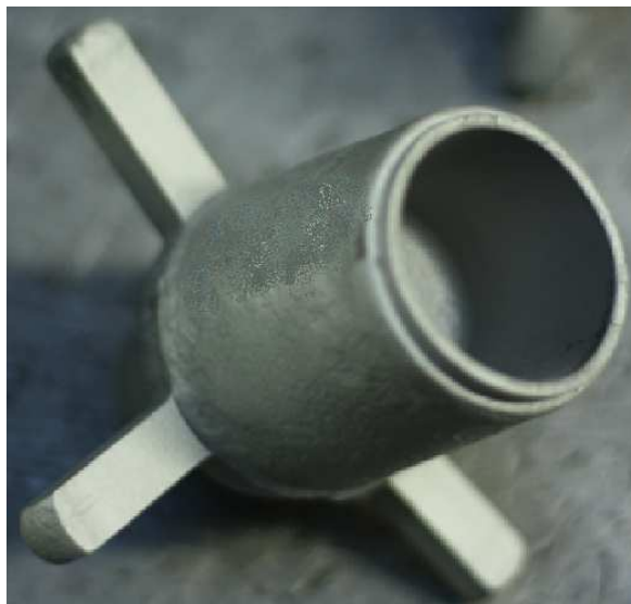
Figure 4: Thixoforged part at 1460^\circ\text{C} in a heated die.
