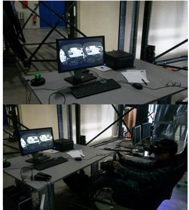
Fig. 1. Oculus rift HMD in driving simulation experiments
