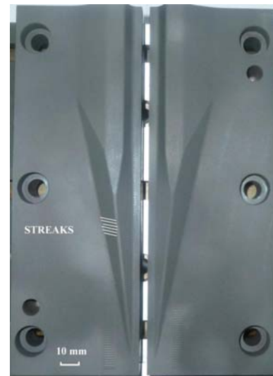
Figure 6. Flat dies used for the experimental tests
