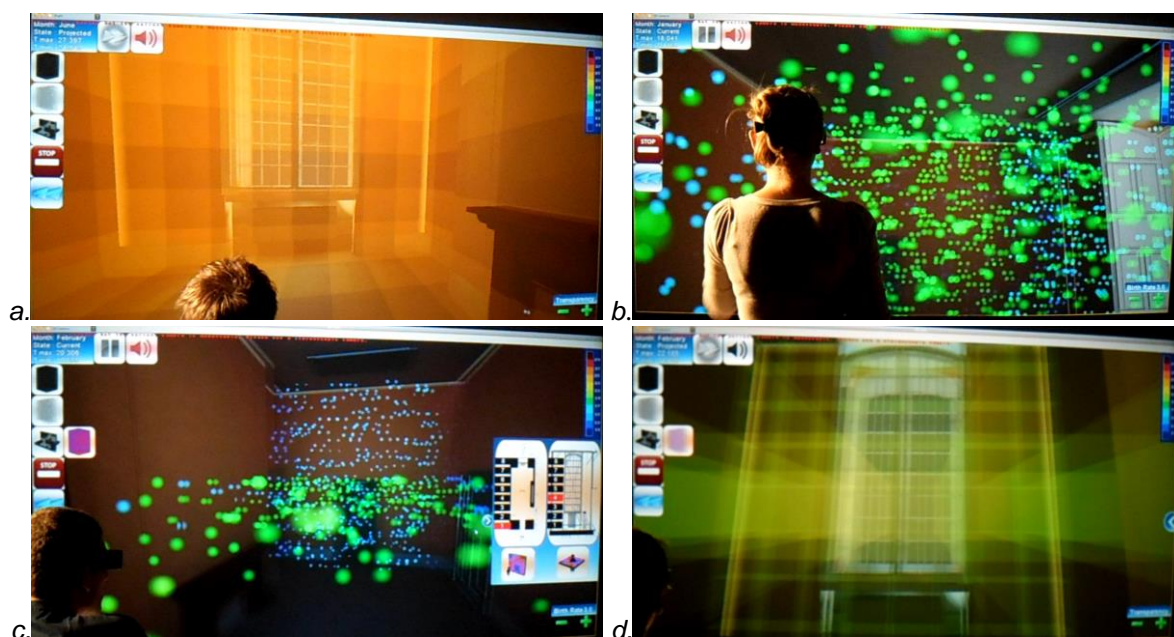
Figure 7. Thermal metaphors of transparent cubes and particles simulated in the immersion room with stereoscopic visualization tested by some participants. (a). Simulation results of renovated version in June 6 th , 14:15 with colored cubes (b). Simulation results of the Gunzo room in existing conditions in January, using particles (c). Simulation results on February 6 th , 14:15, using layer particles in vertical and horizontal (d). Simulation results of the renovated version using layer cubes in vertical and horizontal.
